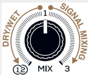
Simply: the left range of the potentiometer acts as a dry/wet for the ring modulator, while the right range allows signal crossfading.
